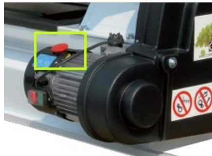
Old style emergency stop button pictured above.
