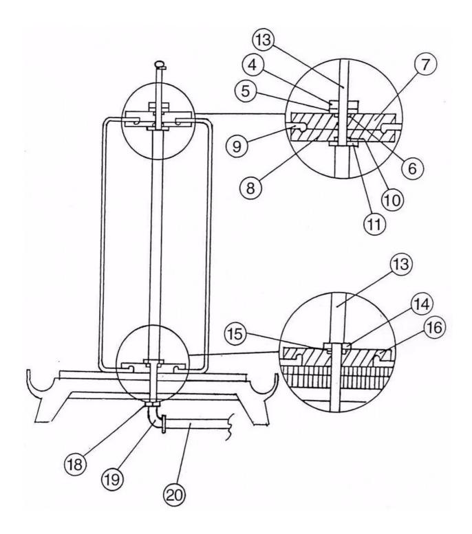
To replace the membrane carefully observe the drawing above and perform the following operations: loosen the lock nut (N°4), remove the washer (N°5), the O-ring (N°6) and the flange (N°7); unscrew the connection pipe (N°20), the bend (N°19) and the lower lock nut (N°18); now remove the shaft (N°13) from the base and replace the membrane.
