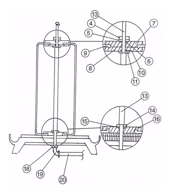
To replace the membrane carefully observe the drawing above and perform the following operations: loosen the lock nut (N°4), remove the washer (N°5), the O-ring (N°6) and the flange (N°7); unscrew the connection pipe (N°20), the bend (N°19) and the lower lock nut (N°18); now remove the shaft (N°13) from the base and replace the membrane.
