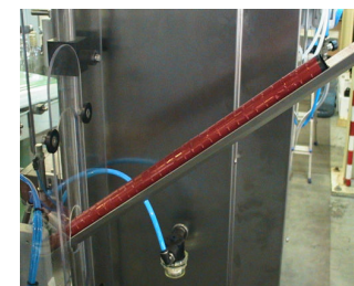
to collocate the capsules on the short pipe
