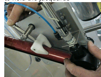
to adjust the capsules in beat at the rotating distributor
